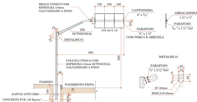
DETALHE DE PLACA SUSPensa EM SEMI-PÓRTICO -ALTA
